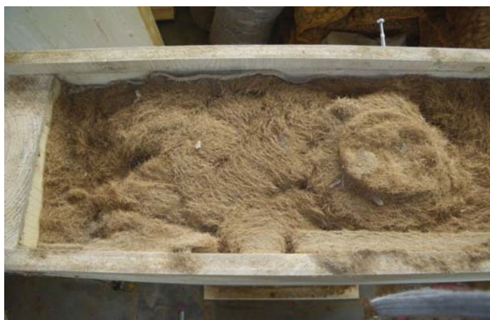
Versatile also in terms of insulation: Zellofant M95 material test with seaweed
